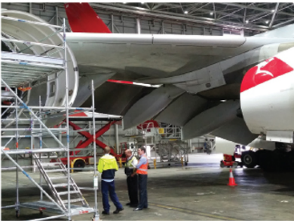
Side Maintenance Stand Lightweight, cantilevered side platforms.
