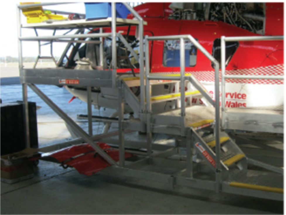
Eurocopter Platforms Adaptable dual-level access for maintenance tasks around the engine bay and lower rear of the fuselage.
