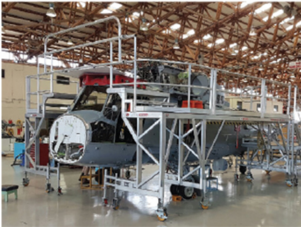
Mobile Docking System Full-Surrounding platform for rotor access with a wide platform for tool storage.
