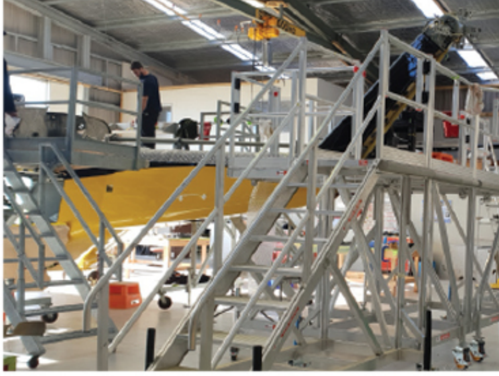
Dual Access Tail Dock Stairs fitted to both sides of platform, for uninterrupted tail access.
