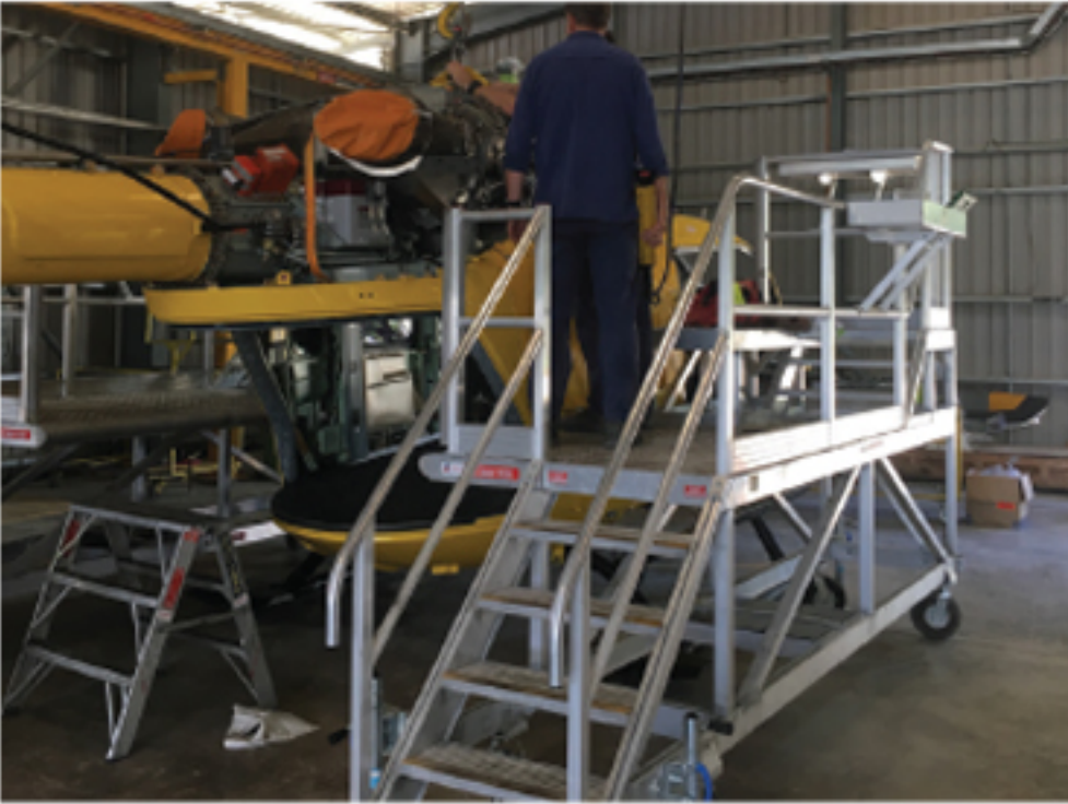
General Service Platform Dual-Level platform for access to main service areas of the aircraft.
